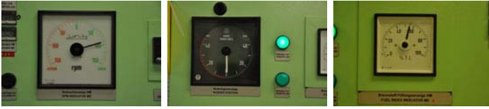
Main engine RPM; Rudder control; Heavy fuel tank level gauge.
