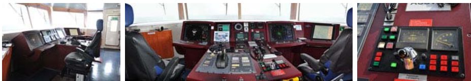
Main command desk: Navigation monitors, main motor and bow thruster control.
