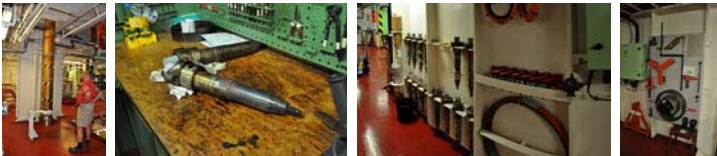
Lower part of a spare piston, fuel injectors and other tools
