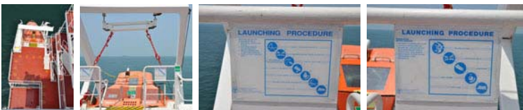
The main live boat can carry 32 people and can be either softly watered or if necessary fast released.
